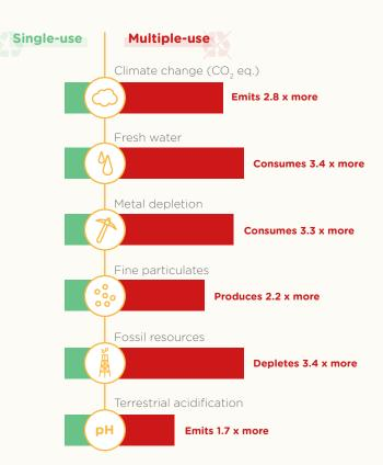
Both systems are equally considered at a 30% recycling rate. Results are similar for a traditional ceramic, glass and metal tableware set, also tested. Multiple-use systems perform better only in ionizing radiation (1.6 times fewer kBq Co-60 eq. to air) and freshwater eutrophication (4.8 times fewer kg P eq.), with only a minimal advantage for ozone depletion. The results represented here are for the baseline scenario.
